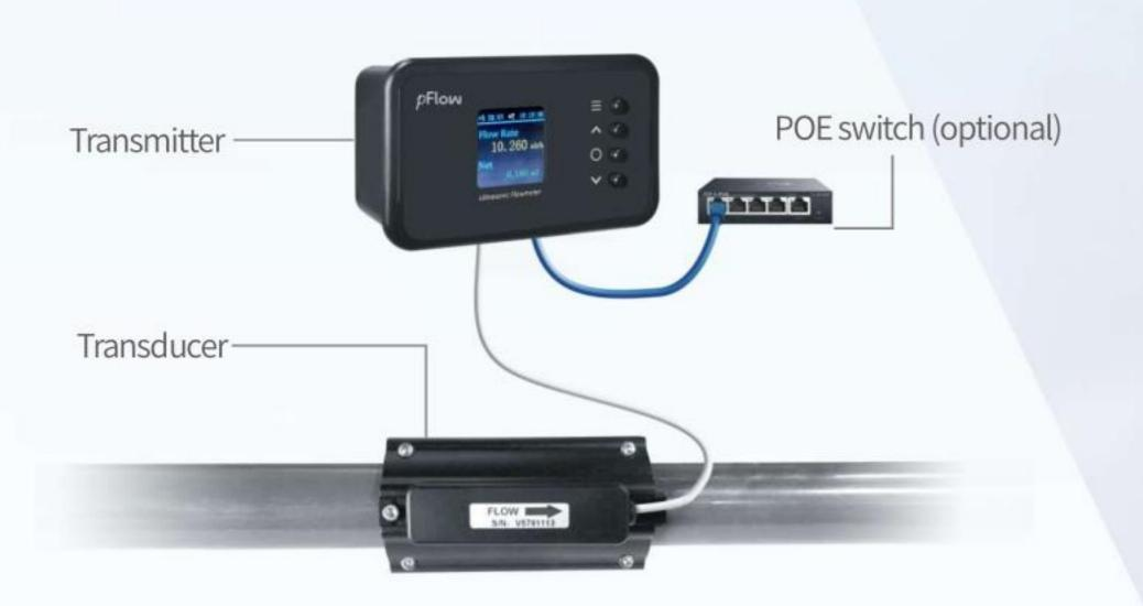
Gentos quick measure ultrasonic flowmeter F3P adopts the measurement principle of transit time method. Combined with Gentos ultrasonic signal processing technology and unique flow algorithm, fluid flow in the pipeline can be accurately measured. The product is designed with a split clamp-on structure, which is simple and convenient to install. The installation process does not need to contact the fluid medium, nor stop production.
